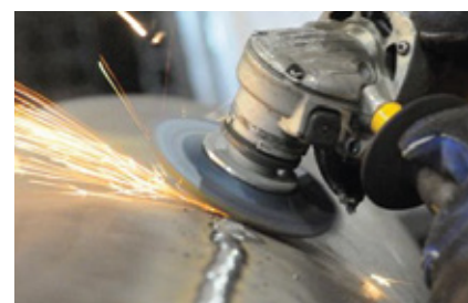
Weld Stock Removal
