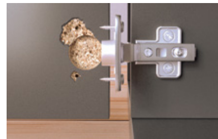
Repairing damaged hinges
