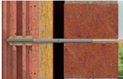
Detail: Repairing outer leaves
