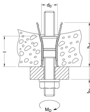
from the anchor collar allowing maximum expansion; it is at this point where the anchor is in contact with the concrete. The shield is divided into four segments so that the load is evenly distributed onto the walls of the hollow section. It is with these characteristics that the anchor expands creating friction and form locking.
