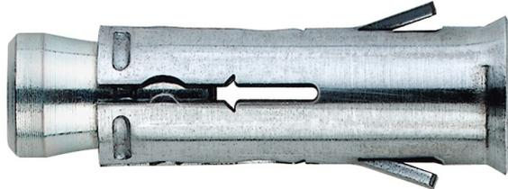
The fischer FHY expansion anchor is the newest anchor from the fischer range. The FHY is designed specifically for hollow-ceiling slabs. The taper section has a continuous internal thread, which permits use with both bolts and threaded rod. The high expansion capacity of the anchor makes it suitable for both solid and hollow-ceiling slabs with a thickness greater than 25mm. The shield of the anchor is 40mm long with sections cut from the shield 21mm
