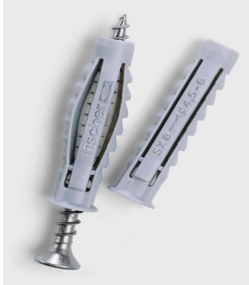
The fischer SX plug has a fourfold nylon plug expansion which form locks with the substrate. This action guarantees maximum load bearing characteristics. The area of application ranges from solid materials through to hollow or perforated materials.
