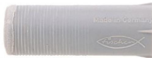
The fischer M Unit is a glass reinforced nylon expansion anchor with an integral internally threaded brass cone. The M Unit expands like a conventional 'Wall Bolt,' but due to the walls of the M Unit being glass reinforced nylon the expansion forces are less aggressive preventing the substrate from crushing during installation. The glass reinforced nylon also reduces noise caused by vibration of pipes, for Mechanical & Electrical applications.
