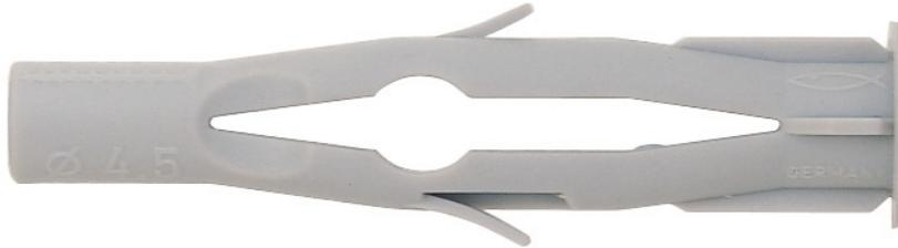
This all round fixing can be installed into almost any kind of substrate, its unique design allows the fixing to expand or to be permanently deformed dependant on the substrate, when installing into a cavity. The rim at the head of the fixing is to prevent it from falling through; the plug is suitable for wood and or chipboard screws.
