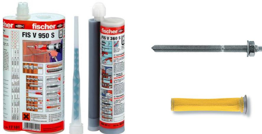
The fischer FIS V injection anchor contains a styrene-free, quick setting, high quality hybrid resin mortar, which is characterized by its universal suitability for many applications. This resin can be used solo or in conjunction with an anchor sleeve dependent on application and substrate. When fully cured this resin produced a form type locking in hollow material and friction type locking in solid material, allowing the application to be a stress free fixing.
