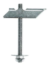
The fischer KD Toggle is the versatile cavity fixing. This fixing can be used in most every kinds of substrate providing it has a cavity, it ranges from M3 to M8 and comes in varying lengths, it is made from mild steel grade 5.8 and is zinc pasivate. The installation procedure is simple and produces very high loads. Smaller versions of the KD toggle come with spring loaded toggle fixing and a selection of threaded attachments from hooks to eyelets.
