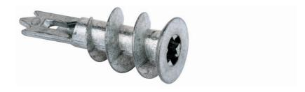
The fischer PDM100 is a self tapping fixing that cuts into the plasterboard until the head is flush with the surface. Installation with a standard Pozi bit means that no special setting tools or pre-drilling is required.
