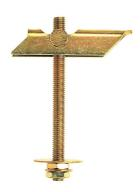
The fischer KD Toggle is a versatile cavity fixing, that can be used in almost every kind of hollow substrate. It ranges from M5 to M8 and comes in varying lengths. The installation procedure is simple and produces very high loads. Smaller versions of the KD toggle come with spring loaded toggles and a selection of threaded attachments including hooks and eyelets.
