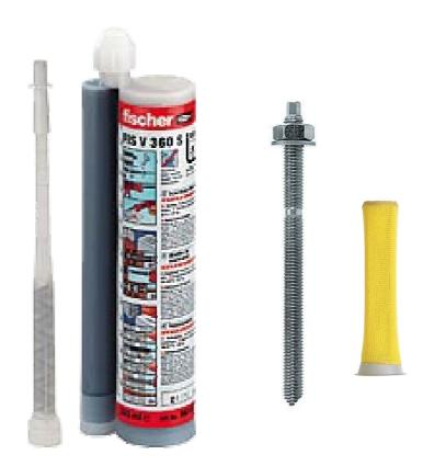
The fischer FIS V injection anchor contains a styrene-free, quick setting, high quality hybrid resin mortar, which is characterized by its universal suitability for many applications. This resin can be used on its own or in conjunction with an anchor sleeve dependent on application and substrate. When fully cured this resin produces a form type locking in hollow material and chemical bond in solid material, allowing the installation to be stress free.
