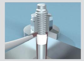
Shear loads with lever arm are not permitted because additional bending will be created which reduces the fatigue resistance of the anchor element. This is also the case, if leveling mortar is used below the baseplate. The max. thickness of leveling mortar without creating bending is  $\leq d/2$  (d = nominal diameter of the fastener) and the compressive strength of the leveling mortar should be  $\geq 30N/mm^2$ .
