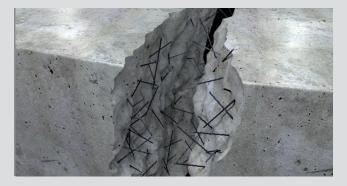
Tests with resin systems, expansion anchors and concrete screws have been performed in SFRC with a steel content of 25 and 60 kg/m<sup>3</sup> by independent institutes to investigate the load bearing capacity and failure mechanism. The series of tests did not show any significant differences between SFRC and normal weight concrete in the failure loads.
