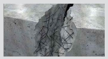
Tests with resin systems, expansion anchors and concrete screws have been performed in SFRC with a steel content of 25 and 60 kg/m³ by independent institutes to investigate the load bearing capacity and failure mechanism. The test series did not
