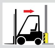
According EN 1991-1-7, design values for accidental actions due to impact from forklift trucks should be determined to take into account the dynamic behavior of the forklift truck as well as the structure. The structural response may
